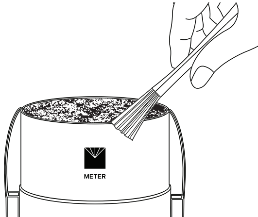
Figure 49 Fix and clean the soil sampling ring
